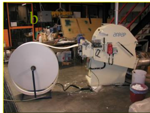
Fig. 3. Open hammer mill (a) and feeding of the material to the hammer mill (b).
