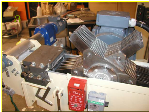
Fig. 3. Open hammer mill (a) and feeding of the material to the hammer mill (b).
