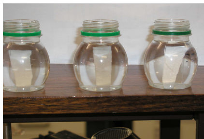
Figure 1 – Picture of the composites specimens immersed in water.
