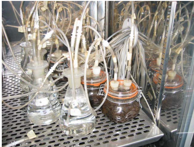
Fig. 1. Reactors for the ultimate aerobic biodegradability tests and humidification flasks.
